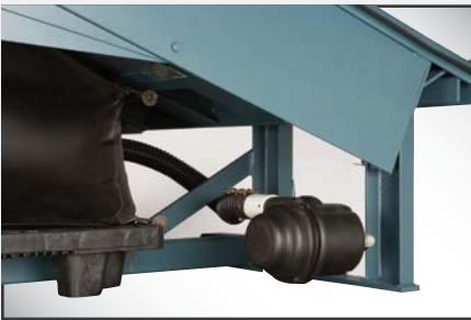
Low pressure 115V/1PH fan motor provides a high volume air supply to reliably activate and position leveler.
