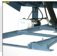
Dual port cylinders allow hydraulic fluid to travel in both directions for a regenerative system.
