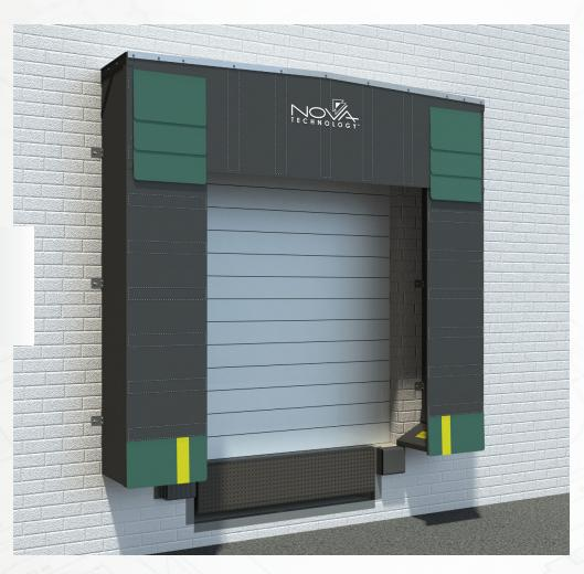
Nova Soft Sided Series Dock Shelter—provides maximum dock protection and full access to trailers while minimizing pressure on the building wall. The Dock Shelter has soft foam sides for added flexibility and is able to compress and bend out of the way of a truck that approaches the doorway off-center or misaligns with the dock. It is designed to be pliable to prevent damage, downtime and costly repairs.
