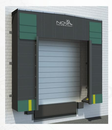
Nova GS Series Dock Shelter—engineered for use with swing-door trailers, the GS Dock Shelter seals the air and light gaps at door hinges while still allowing full access into the trailer. This shelter provides maximum dock protection while minimizing pressure on the building wall. Utilizing foam side pads in its construction, the shelter is capable of compressing and bending out of the way of a truck that approaches the dock off-center preventing costly repairs.
