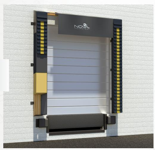
Nova Curtain Head/Side Pads Series Dock Seal—features a hood-style head curtain in place of a head pad with a metal pipe and fiberglass stays in the fabric hood to maintain support and serviceability.
