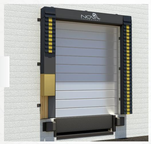
Nova Full Pad Series Dock Seal—the foam-filled head pad and side pads provide a tight, energy-efficient seal between the trailer and dock wall providing protection from inclement weather, dirt and insect infiltration.
