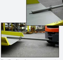
The "Tow Clamp" connects between the ramp pocket and the tow hitch of your fork truck and permits easy transportation of the lift over longer distances.
