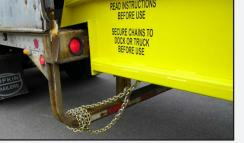
Safety chains hold the ramp tight to the carrier and assure adequate lip purchase is maintained with the carrier bed.
