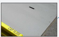
A 60" transition at grade and 30" transition at dock height is constructed of high strength diamond tread plate beveled and recessed for smooth transition onto and off the yard ramp.
